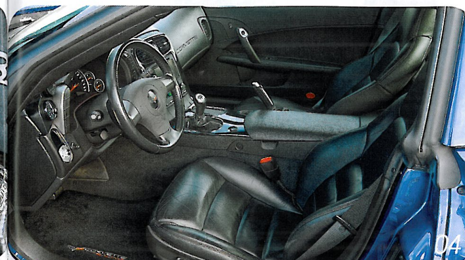
04 → In contrast to the heavily customized engine bay, the interior remains largely stock. Note the Blitz boost controller mounted in the left A/C vent. 05 → Is it a base C6, a Z06, or something else? Bulged rear quarters and a lip spoiler from the latter model make it difficult to tell.
