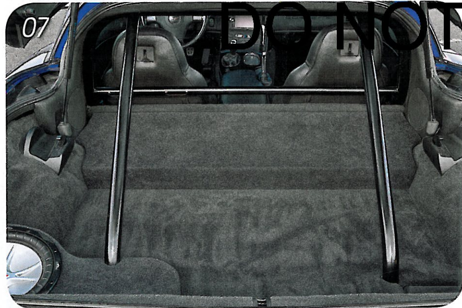
06 → Transplanted Grand Sport fenders and six-pot Z06 brakes further confound would-be model spotters. 07 → Four-point rollbar seems a prudent addition in light of the car's projected 230-mph top speed.
