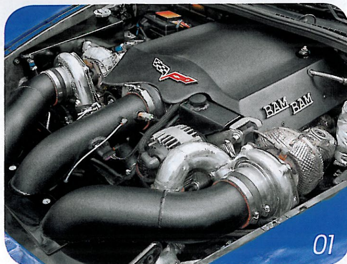
01 → Twin 78mm ball-bearing turbos ram up to 28 psi of boost down the 427-cube Superdeck engine's gullet. With more than 1,400 dyno-destroying rwhp available, the "Bam Bam" sobriquet is an appropriate one. 02 → Heat shielding is deployed liberally
