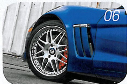
06 → Transplanted Grand Sport fenders and six-pot Z06 brakes further confound would-be model spotters. 07 → Four-point rollbar seems a prudent addition in light of the car's projected 230-mph top speed.
